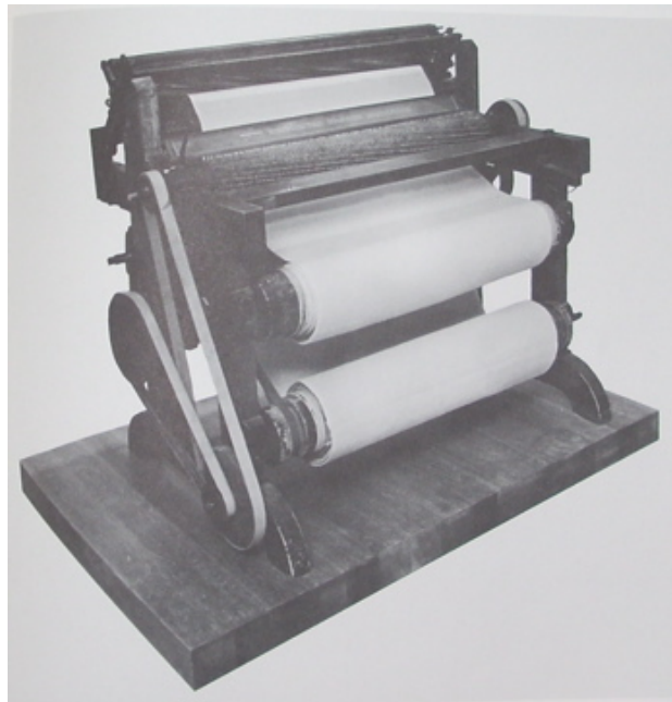
Figure 3.15. Rotary shear from 1840. New Yorker Samuel Dorr patented the first rotary shear in 1792. From Homespun to Factory Made: Woolen Textiles in America, 1776-1876 , p. 97.
