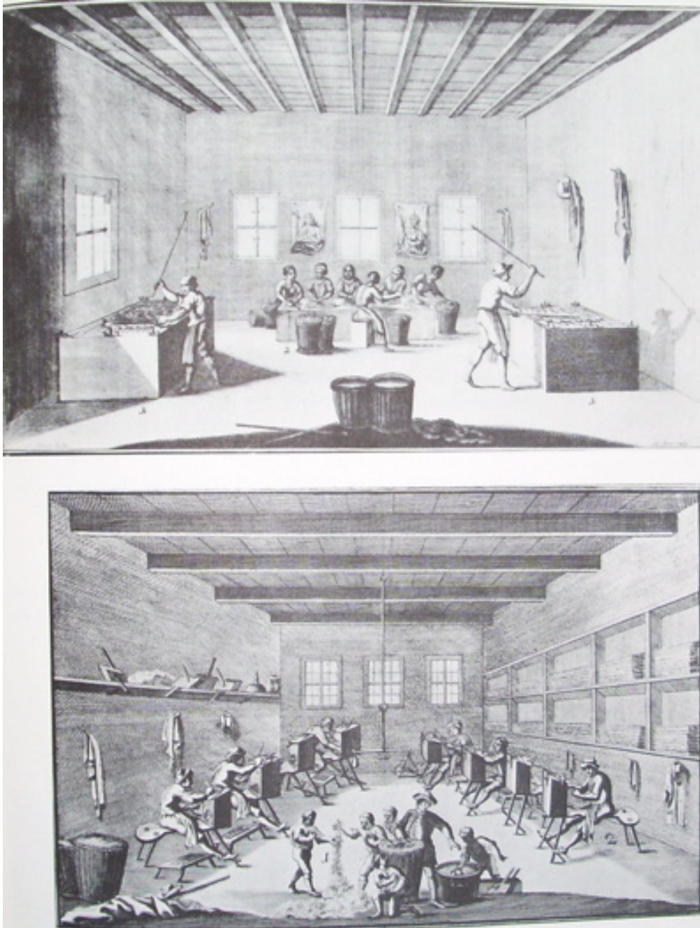
Figure 3.7. Picking removed the dirt, dung, straw, and other impurities from the scoured wool. Pickers spread wool on a clean floor, then beat it with sticks to knock the debris loose, which was subsequently collected and discarded. From Homespun to Factory Made: Woolen Textiles in America, 1776-1876 , p. 15. Images from The Waldstein Woolen Mill by Freudenberger, Plates 8 and 10.
