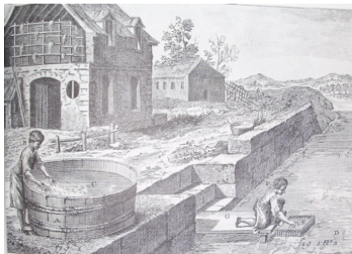
Figure 3.6. After sorting, scouring was performed on the raw wool, in which the lanolin and suint, the wool’s protective substances, were removed by immersing it into a mixture of stale urine and water, then rinsing it with fresh water, and drying it on a rack. From Homespun to Factory Made: Woolen Textiles in America, 1776-1876 , p. 13. Image entitled “Draperie,” Plate I, Fig. 1, from Denis Diderot’s Encyclopedie, Recueil de Planches , vol. IV. Paris, 1763.
